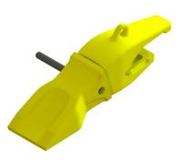
**4) Insert Pin:** Insert the pin - recess end first - through the tooth and adapter from the opposite side of the retainer.
