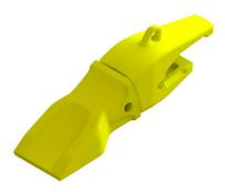
3) Install Tooth: Position the tooth on the adapter, ensuring the retainer does not fall out.
