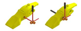
**Pin Removal:** Remove the existing CAT bucket teeth by using Cutting Edge's pin removal tool (part number 7013). Hammer the pin removal tool into the pin from the side of the tooth with the retainer. Once the pin has been removed, the tooth can also be removed from the adapter.
