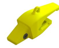
2) Install Retainer: Prior to install, ensure both the tooth and adapter are clear of any dirt. If not, then clean using a wire bristle brush or equivalent. Apply silastic to the back face of retainer prior to installation to hold it in place and then position the retainer into the recess of the adapter.
